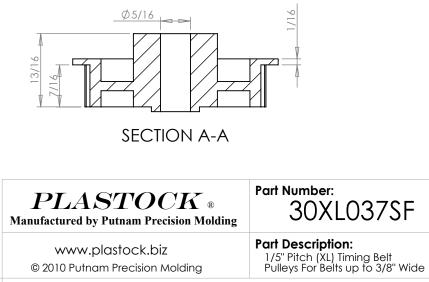
Dimensions are in inches Tolerances: Fractional ± 0.015 The INFORMATION CONTAINED IN THIS DRAWING IS THE SOLE PROPERTY OF PUTNAM PRECISION MOLDING. ANY REPRODUCTION IN PART OR AS A WHOLE WITHOUT THE WRITTEN PERMISSION OF PUTNAM PRECISION MOLDING. MOLDING IS PROHIBITED. INFORMATION IN THIS DRAWING IS PROVIDED FOR REFERENCE ONLY.
